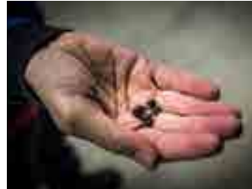
Crushed Filtralite used as a filter at VEAS.
