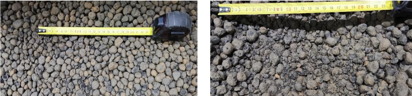
Figure 32.- Left: LECA material at the top of layer, no breakage. Right: LECA material broken at some centimetres below top surface
