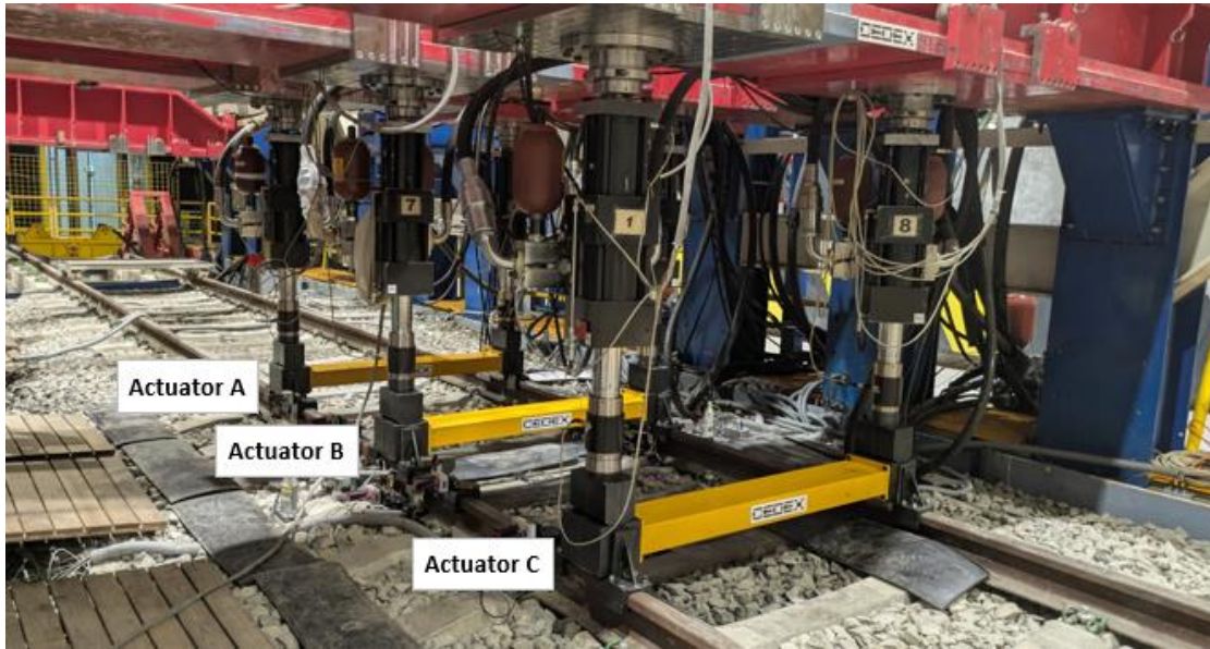
Figure 57.- Hydraulic actuators disposition in CTB
