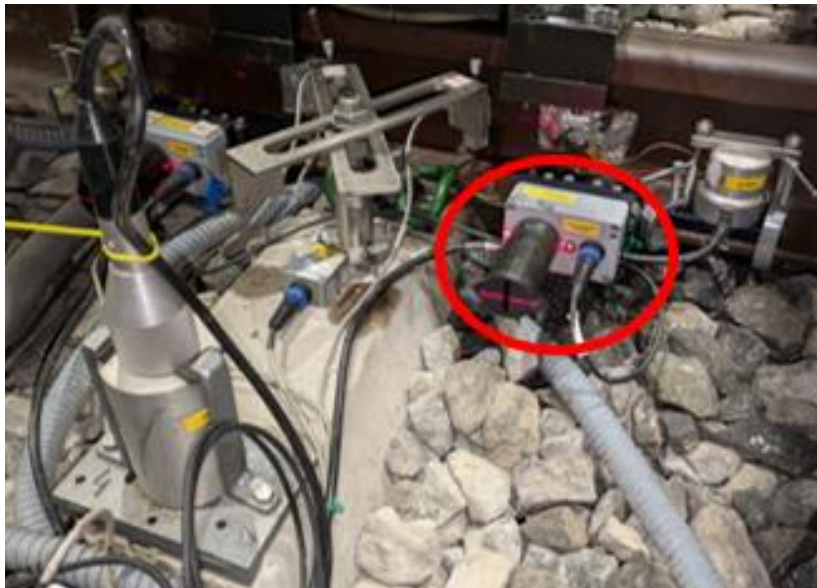
Figure 75.- Detail of the laser system used to measure the vertical displacements of the railway track section
