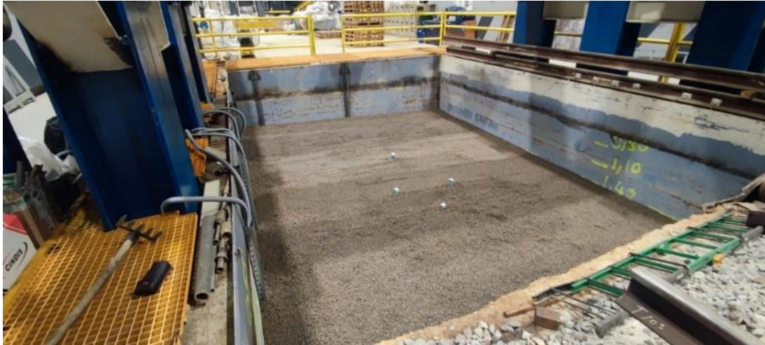
Figure 29 General view of test section with LECA layer once compacted and finished
