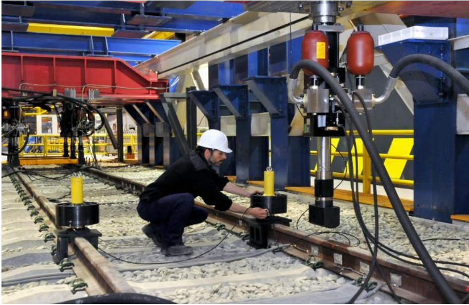
Figure 8.- Piezoelectric actuators to simulate the effect of track imperfection
