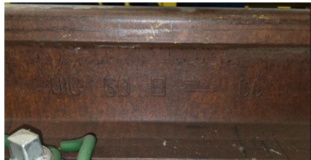
Figure 17: UIC 60 rail used in railway track section
