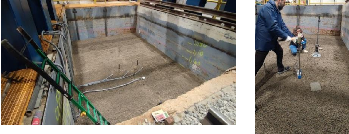
Figure 26.- Left: Aspect of the test section with the half-thickness of LECA embankment, in which some instrumentation was already installed. Right: Execution of Panda test in the half-thickness of LECA embankment. The dynamic load plate is shown in the background
