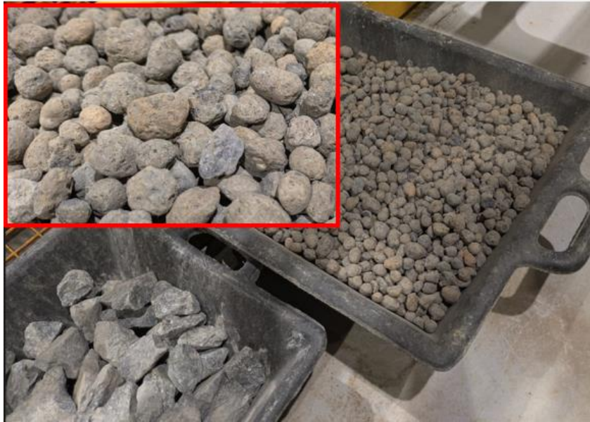
Figure 12.- Appearance of LECA material (10/20) used in the railway track section
