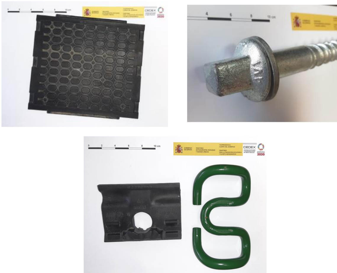
Figure 18.- Fastening system components:Up-left: Under-rail pad; Up-right: Screws; Down: Angular guide plate and clip
