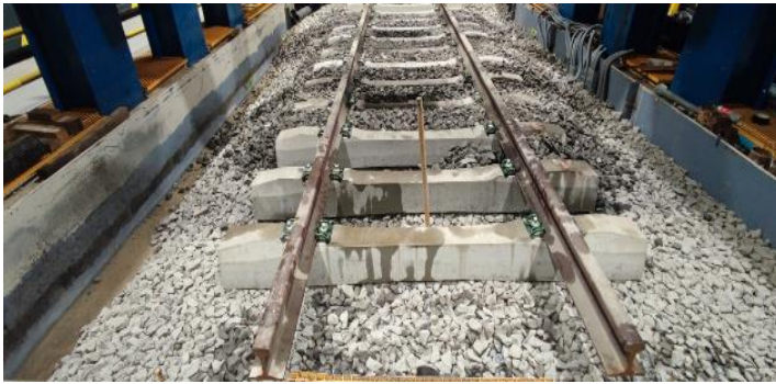
Figure 43.- Left: Ballast layer with sleepers, rails and fastening system. Right: Hand-held vibrator for ballast compaction
