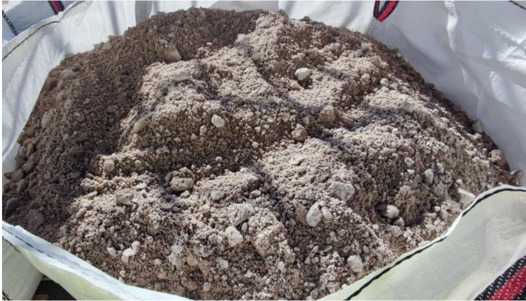
Figure 14.- Granular sub-ballast used in the railway track section
