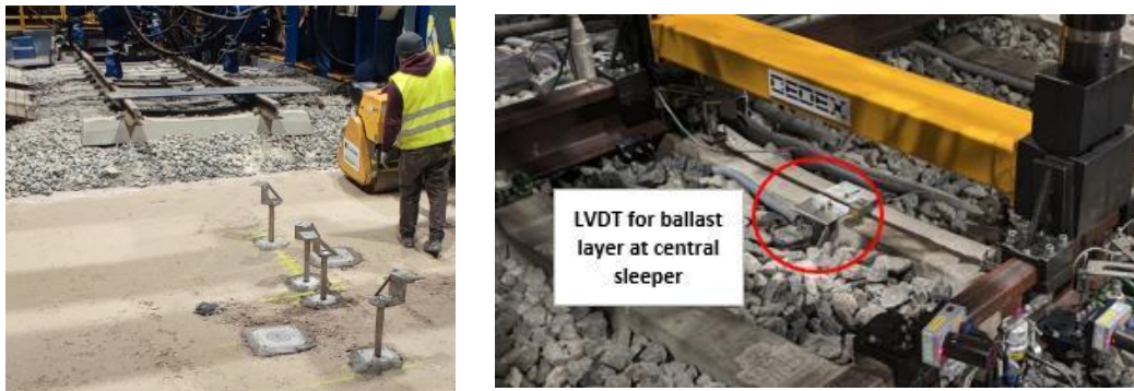
Figure 87.- Instrumentation for ballast displacement measurement. Base of LVDT fixed at the top of the sub-ballast layer (left). Head of LVDT fixed at the sleeper (right).
